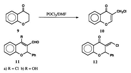
Under analogous conditions after 80 hrs, the reaction mixture did not contain the flav-3-ene **11a** but two new products were observed by TLC. Separation of this mixture by means of column chromatography then resulted in the isolation of (3-formyl-4-hydroxy)flav-3-ene **11b** and 3-chloromethyleneflavanone **12** in pure form. Further transformations of **2a-e** are in progress.
